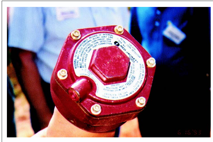
Line Leak Detector Flow Restrictor ("Red Jacket"), or Flow Shutoff, or Alarm System
