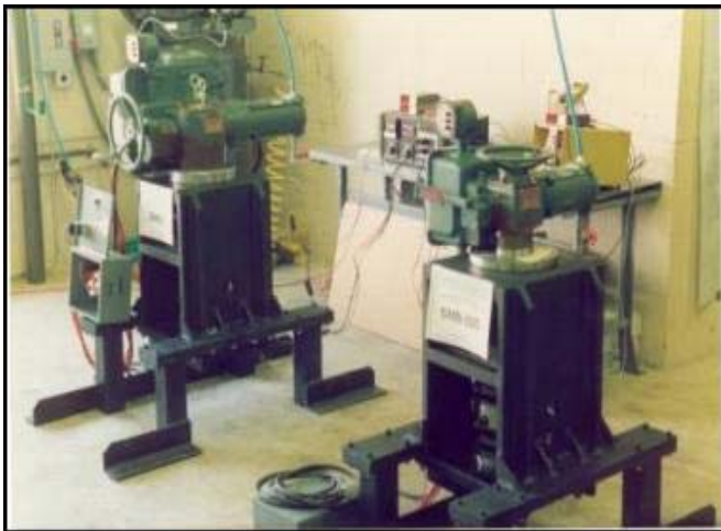
Figure 2 - Test Fixtures Used for Cyclic Testing of Limitorque SMB-000 through SMB-1 Actuators (shown on the left). A higher load capacity test fixture (shown on the right) was used for SMB-2 Testing
