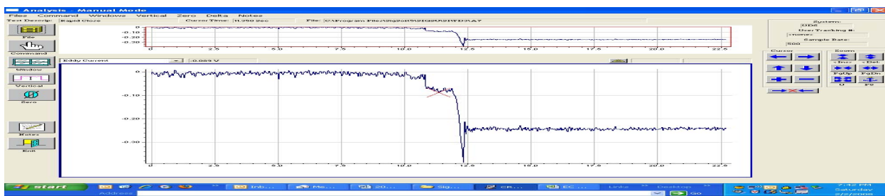
NIC Phase 4 Trending TD3 eddy current data for swing check valve closing stroke test with 50% worn hangar arm degradation. Notice the abrupt change in negative stroke delta as a result of the excessive clearance when the disc seats.
