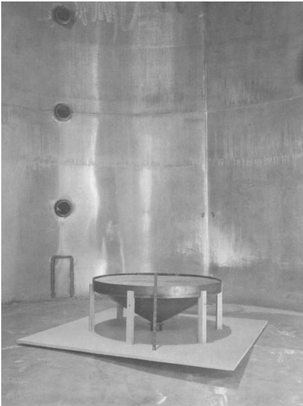
Figure A.42. Stainless Steel Screen and Support Used in Burining of Flammable Materials
