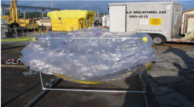
Exhibit 4-20: Sleever containment for jumpers.
