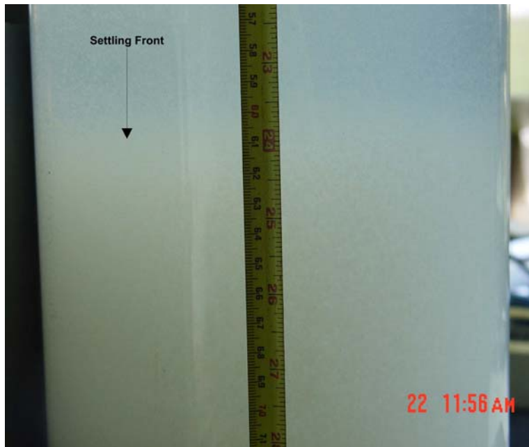
Figure 20. Settling front in test with 300 ppm Cl
