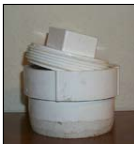
d. The gravel sampler. Note beveled edge on bottom of sampler to improve coring.
