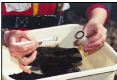
b. Preparing to scrape a rock using the SG-92 sampler (showing o-ring) and periphyton brush.
