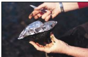
c. Foil covering the scraped area of a rock following the top-rock scrape method.
