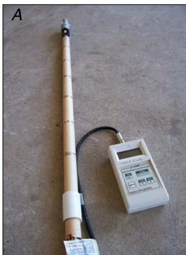
Light meter and sensor disk with sensor cord running through a graduated PVC pipe. The light-sensor disk is taped so it is facing upward on the measuring rod.
