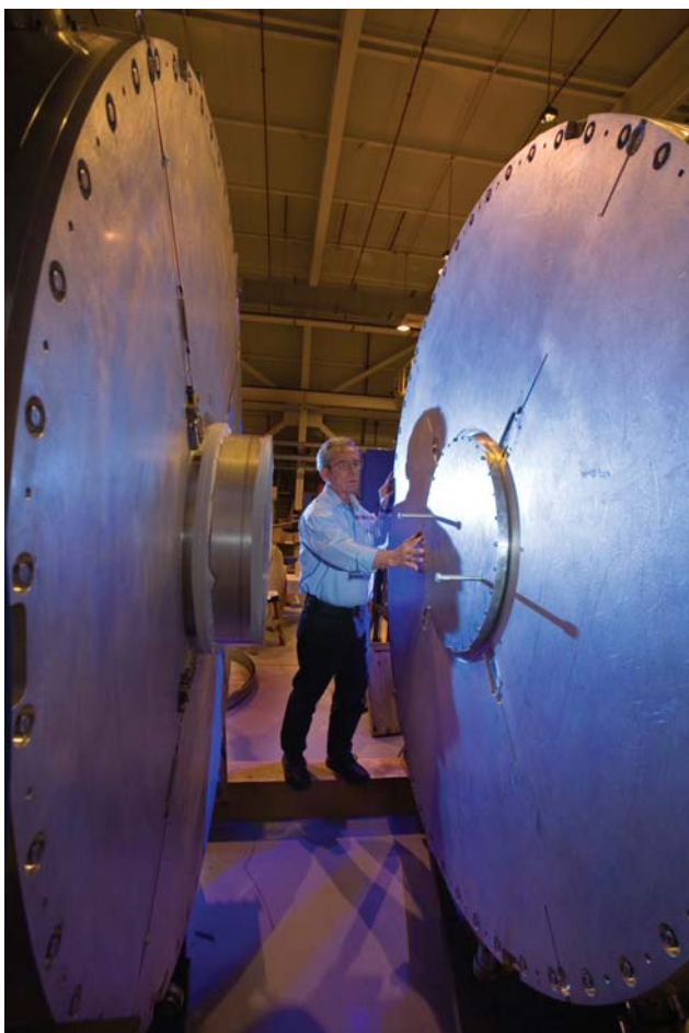
DIGITAL IMAGE MAKER: DARHT uses these large circular aluminum structures to create magnetic fields that focus and guide a stream of electrons down the length of the accelerator. The final product of the process is images of mock nuclear devices as they implode.
