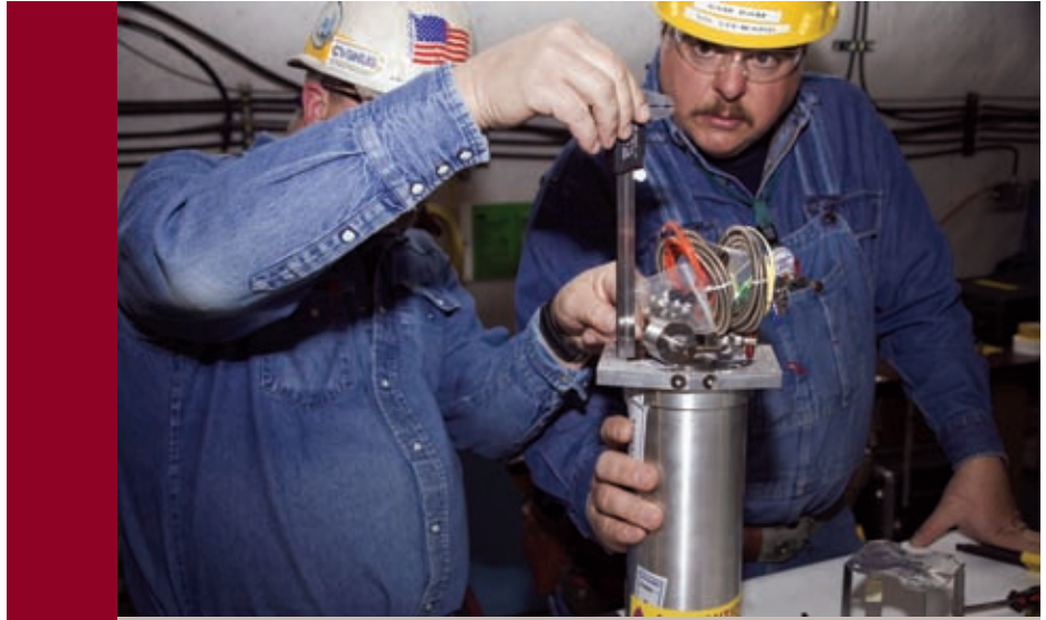
PU EXPERIMENT: Technicians prepare a dynamic plutonium experiment, named Thermos, at the U1a facility 1,000 feet underground at NNSA's Nevada Test Site. The Thermos experiments are designed to study damage to plutonium under dynamic loading conditions.
