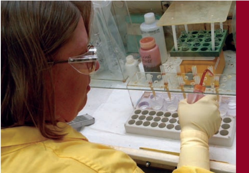
ENSURING QUALITY: A technician prepares the solutions for analysis of chemical composition. This ensures that the material meets quality requirements for entry into the U.S. nuclear weapons stockpile. See pages 4 and 5 for more on Los Alamos National Laboratory's completion of the first war-reserve quality plutonium pit.
