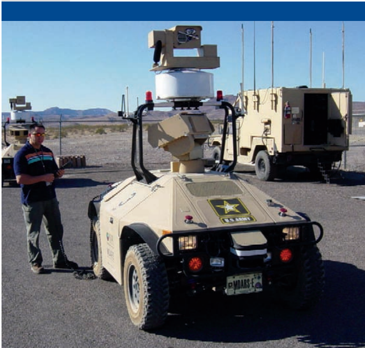
ROBO SECURITY: A mobile detection and reconnaissance vehicle is shown being tested at the Nevada Test Site. These robotic systems are currently in use by the Army and are being evaluated for use to augment existing security forces throughout NNSA. These robots have the ability to detect intruders at great distances and provide security forces with the exact locations and number of intruders being monitored.
