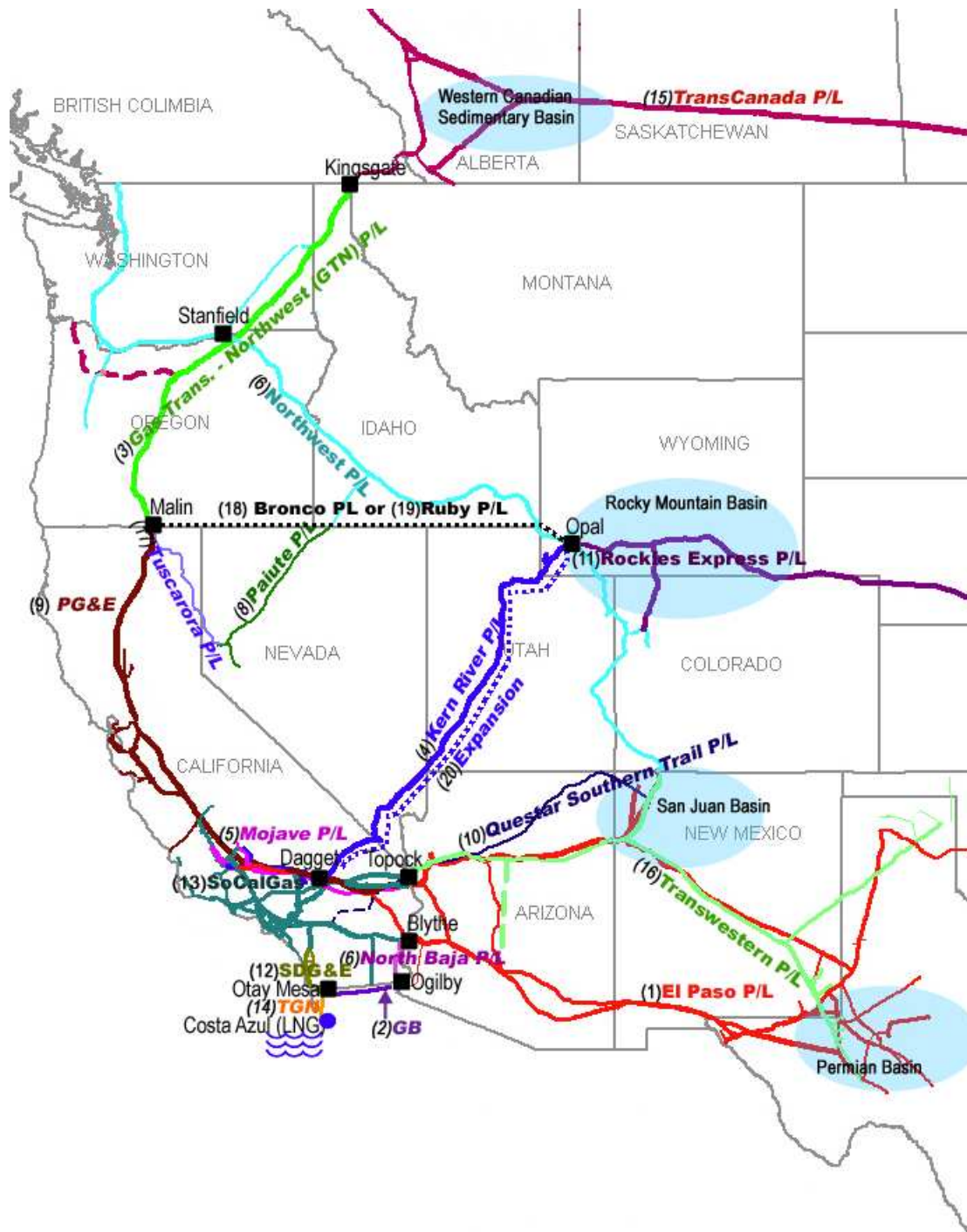
Figure 3 - Western North American Natural Gas Pipelines
