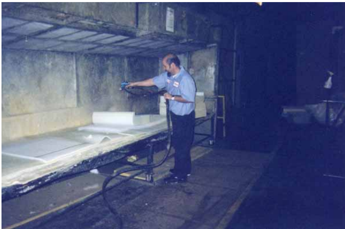
Figure 3-8. Adhesive Spray Booth at Hickory Springs.
