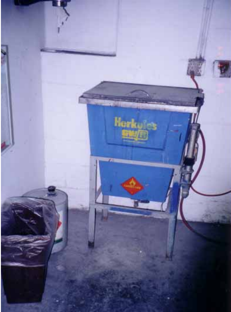
Figure 3-6. Spray Gun Cleaning System at Westway.
