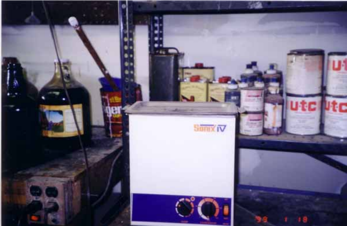
Figure 3-4. Tabletop Ultrasonic Cleaning Unit at Bausman & Father.
