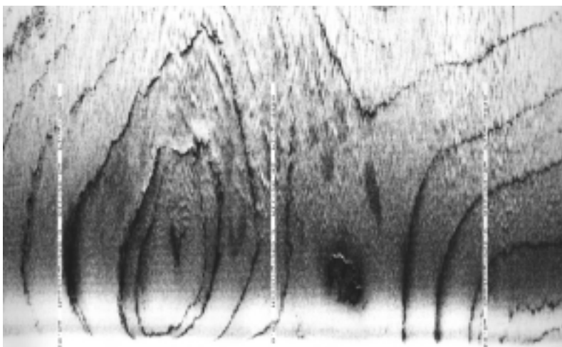
USGS side-scan sonar record north of Anacapa Island, June 1998. This is a one square kilometer image of the seafloor surface. Dark areas indicate hard rock layers, while lighter areas show softer rock. The tree-ring pattern on the sea floor is the result of wave erosion.
