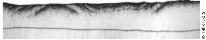
USGS side-scan sonar record north of Anacapa Island, June 1998. This sub-seafloor layer image is a geologic structural profile of the ocean bottom down to about 30 meters. The sub-floor profile reveals the thickness of sediment types over bedrock.
