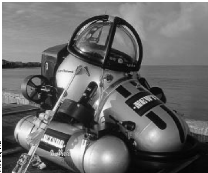
DeepWorker 2000 consists of a sphere where the pilot sits with an attached cylinder (for the pilot’s legs) and a Plexiglass viewing dome. The sub weighs just over 2,000 lbs with a total payload of 250 lbs, including the pilot.
