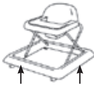
Newer style has a gripping mechanism under the edge to stop the walker at the edge of a step
