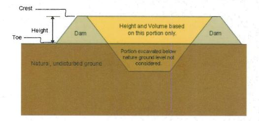
**NOTE:** On slopes, the height of the dam should be measured from the downhill or downstream toe of the dam to the lowest point on the crest of the dam.
