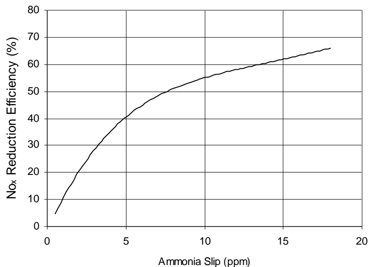
Figure 1.7: \text{NO}_x Reduction for Various Ammonia Slip Levels
