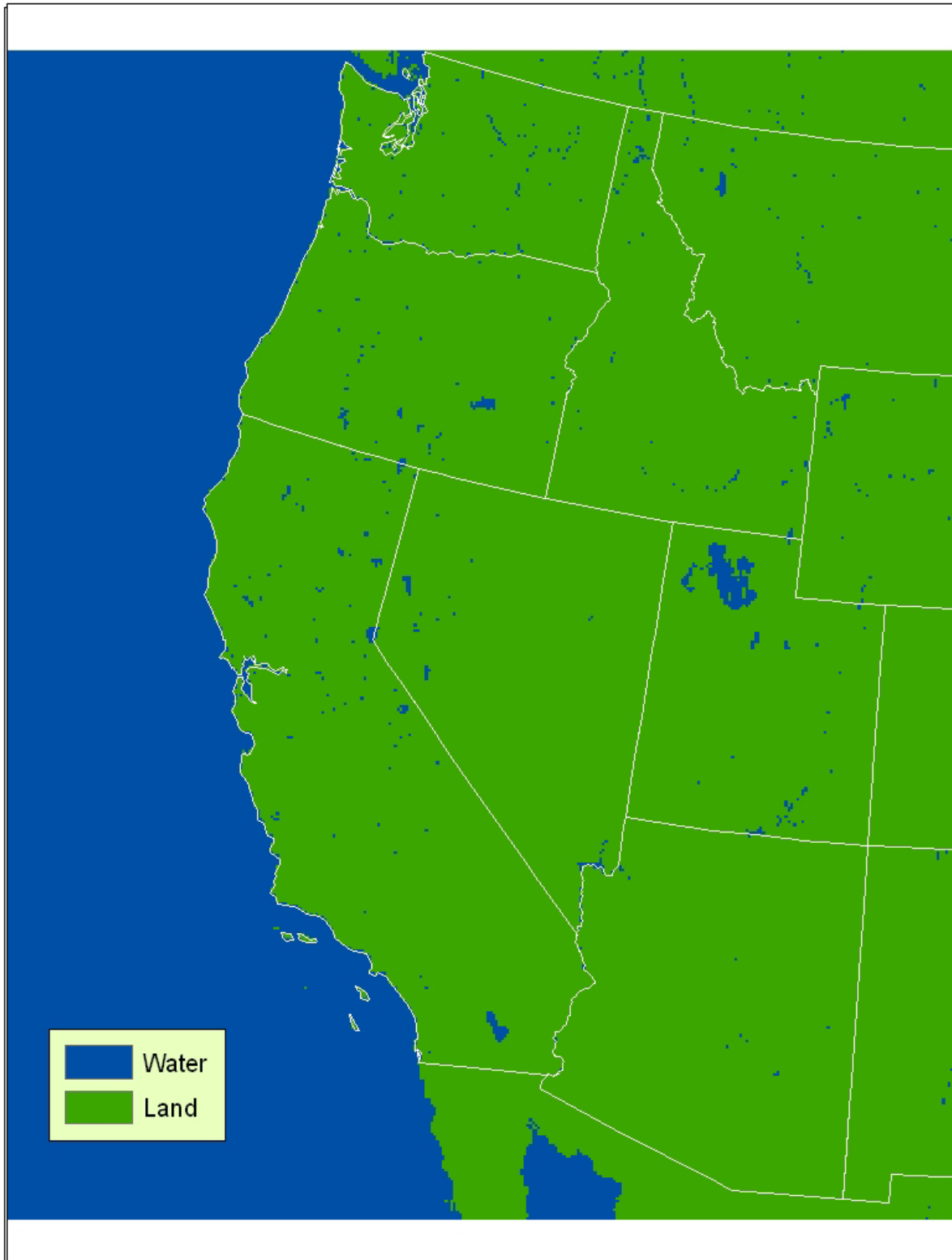
Figure 5. The 5-km land water masks developed from the 1-km GLCF land cover data. These data are the foundation of the station designations discussed later in the paper.
