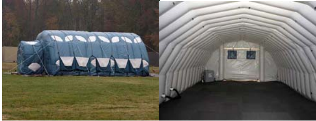
Figure 11. The inflatable habitat produced as part of an FY 2006 Seed Fund project, prior to its trip to Antarctica for testing at the NSF McMurdo Station.
