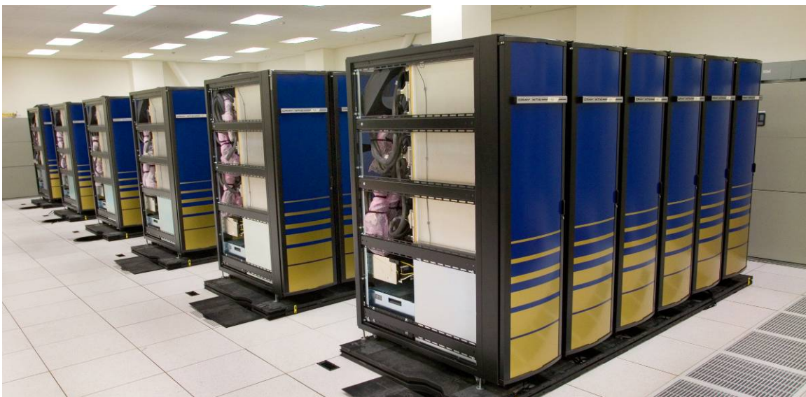
Figure 14. The first 36 cabinets of NERSC’s Cray XT4 supercomputer, which, when complete, will deliver sustained performance of at least 16 teraflop/s.
