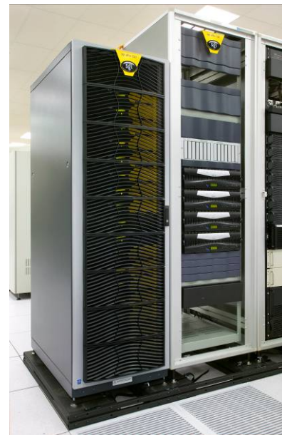
Figure 13. DaVinci is a 32-processor SGI Altix with 6 GB of memory per processor and 25 TB of disk memory, a configuration designed for data-intensive analysis and interactive visualization.
