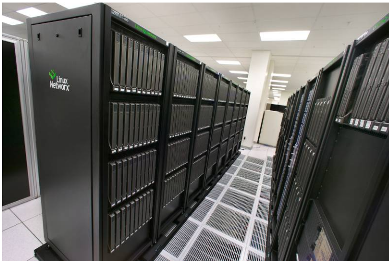
Figure 11. Jacquard is a 722-processor Linux Network Evolocivity cluster system with a theoretical peak performance of 2.8 teraflop/s.
