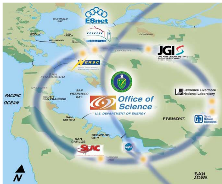
Figure 15. ESnet's new San Francisco Bay Area Metropolitan Area Network provides dual connectivity at 20 to 30 gigabits per second to six DOE sites and NASA Ames Research Center.
