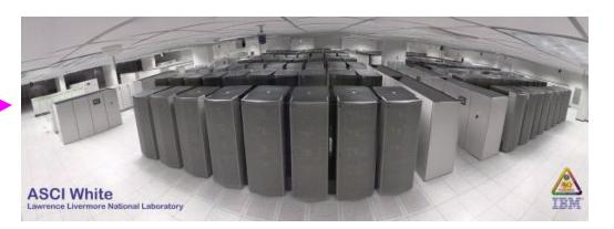
Clusters of Symmetric Multiprocessors: Ensembles of Data Servers + Fast Switch
