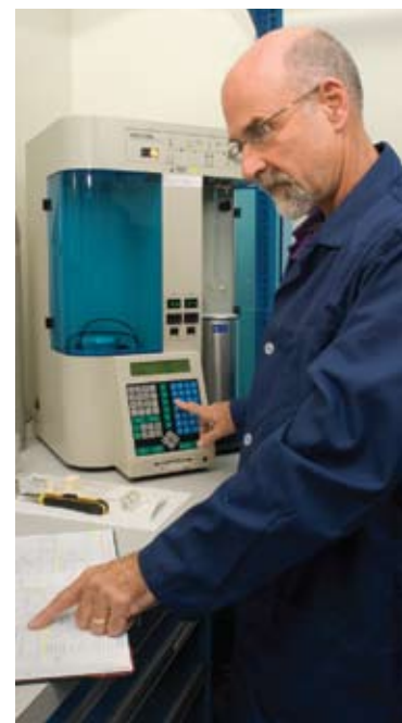
Barry Meneghelli performs surface area analysis of an aerogel material.
