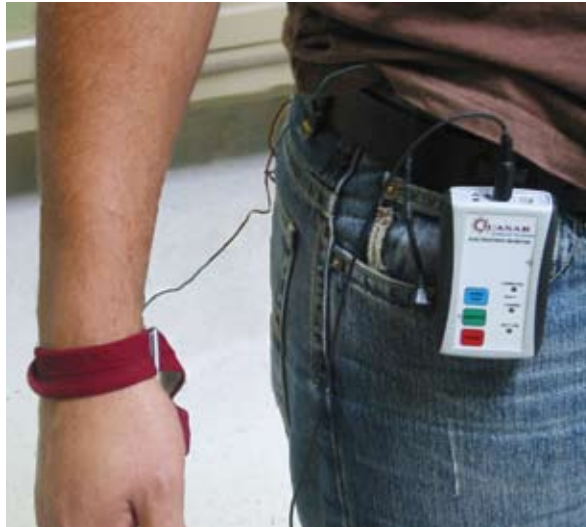
The lightweight Remote Voltage Sensor enhances personnel safety and device protection. (photo courtesy of QUASAR Federal Systems, Inc.)
