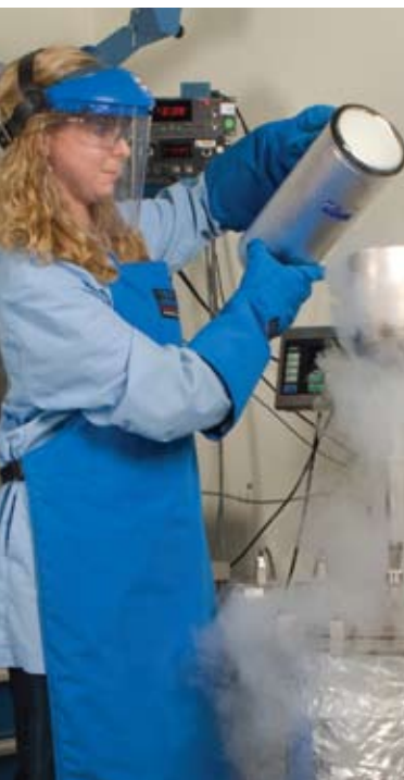
Brekke Coffman fills the Cryostat-4 with liquid nitrogen to test new insulation systems for future space exploration missions.
