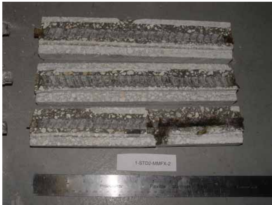
Figure 4.59. Photo. Trace of the upper rebars and corrosion products on specimen number 1-STD2-MMFX-2.
