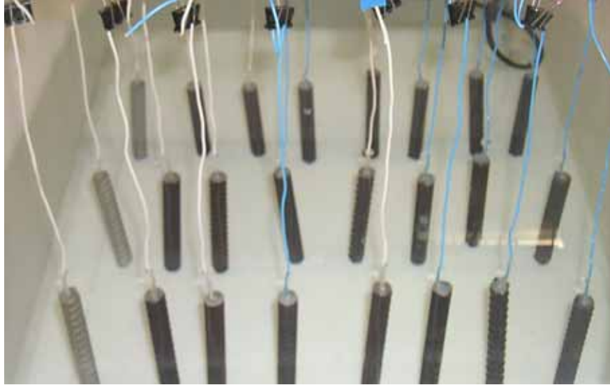
Figure 3.6. Photo. AST-1 specimens under test in the upper hold tank (figure 3.5).
