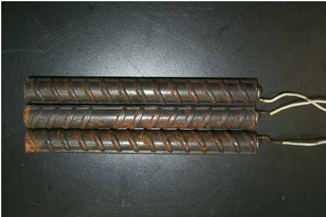
Figure 4.13. Photo. MMFX-II™ specimens subsequent to AST-1 testing.
