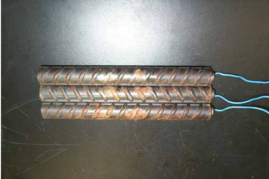
Figure 4.14. Photo. MMFX-II™ abraded specimens subsequent to AST-1 testing.
