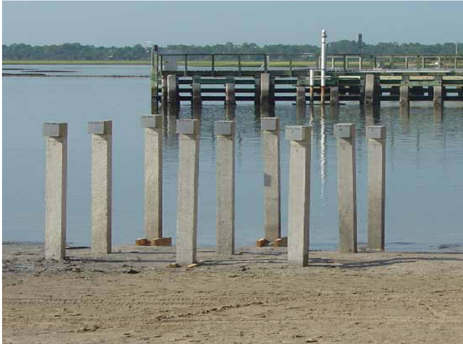
Figure 3.27. Photo. Field column specimens under exposure at the Intracoastal Waterway site in Crescent Beach, FL.
