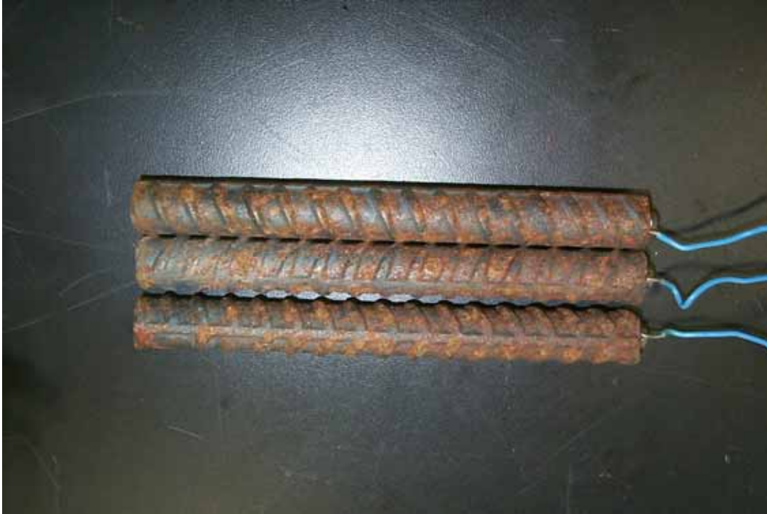
Figure 4.16. Photo. Black bar specimens subsequent to AST-1 testing.
