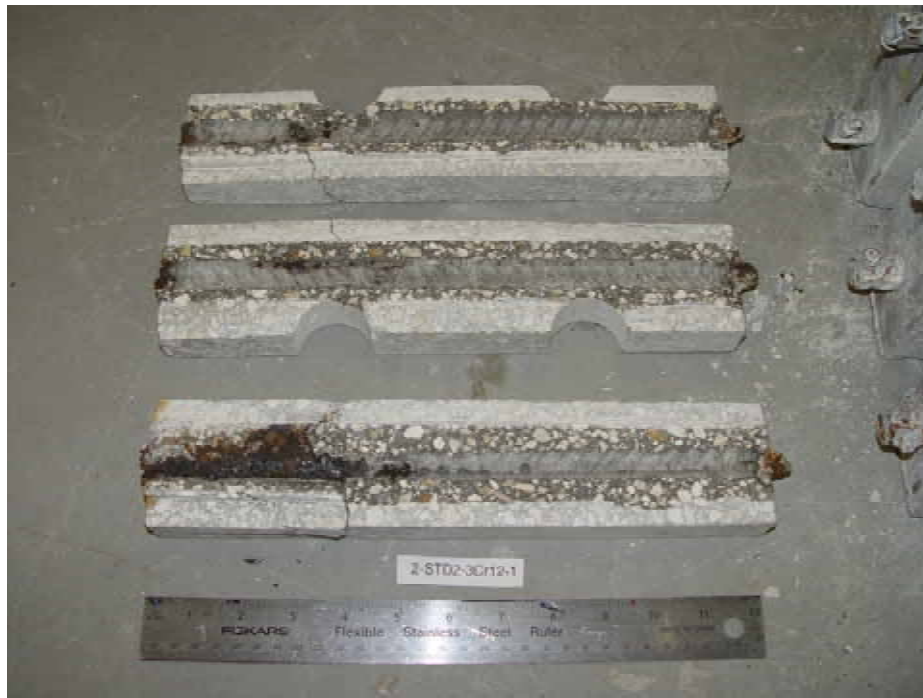
Figure 4.82. Photo. Trace of the upper rebars and corrosion products on specimen number 1-STD2-3Cr12-1.
