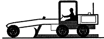
3. Windrow Existing Asphalt Bound Materials
