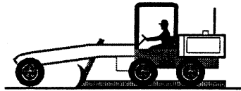
3. Windrow Existing Asphalt Bound Materials
