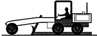
3. Windrow Existing Asphalt Bound Materials
