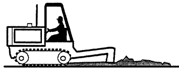
1. Rip and break existing pavement
