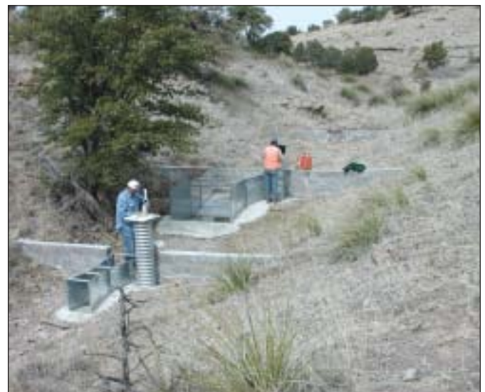
Scientists installed Parshall flumes and a sediment dam in New Mexico to test the effects of spring and summer prescribed burns on oak savanna ecosystems.
