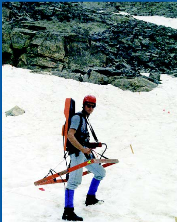
Figure 18 – EMI skirt configuration. Photo courtesy of Blackhawk Geometrics.
