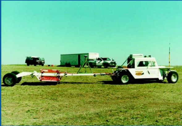
Figure 16 – MTADS configured with EMI sensors. Photo courtesy of Blackhawk Geometrics.
