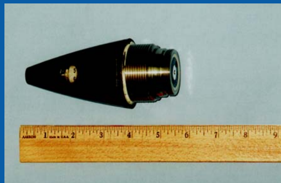
Figure 32 – The numbers in the “window” of this fuze for a 155 mm projectile indicate an internal timing mechanism to allow for an airburst of the projectile.
