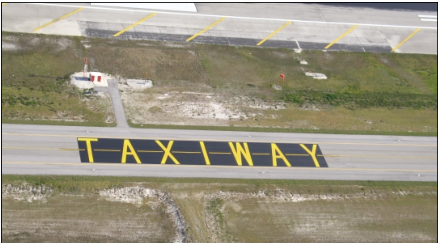
Taxiway "L" is located between Runways 9L/27R and 9R/27L. Taxiway "L" is now clearly marked to help prevent future errors.
