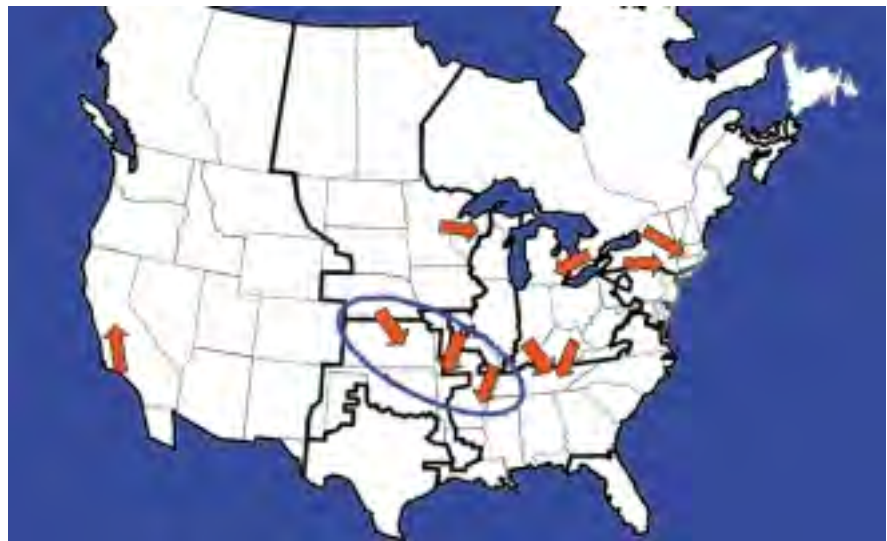
Figure 7-2 Current Electric Power Bottlenecks
