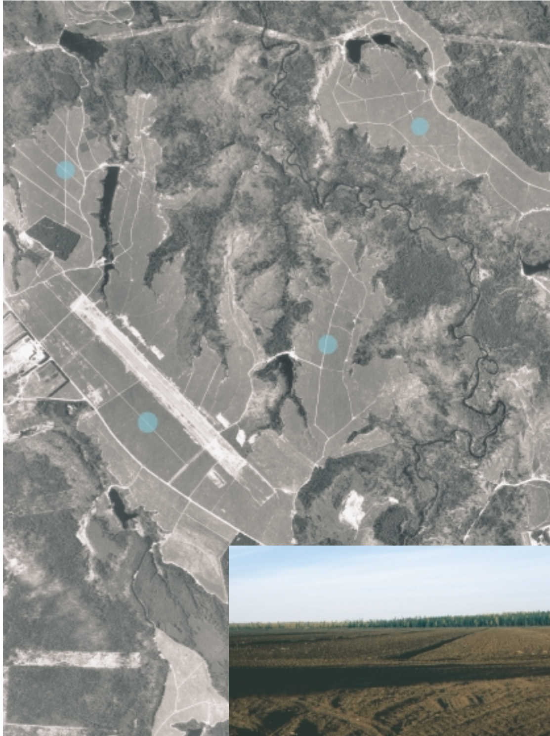
Figure 41. A black-and-white aerial photograph of peat extraction (mining) in Maine, 1996. The areas indicated by a blue dot in the center have had the surface vegetation removed, but they remain wetland. The accompanying color photograph shows the peat surface. (Aerial photograph: National Aerial Photography Program)
