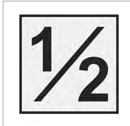
FIG ENR 5.7-1 Typical Runway Half-way Sign
