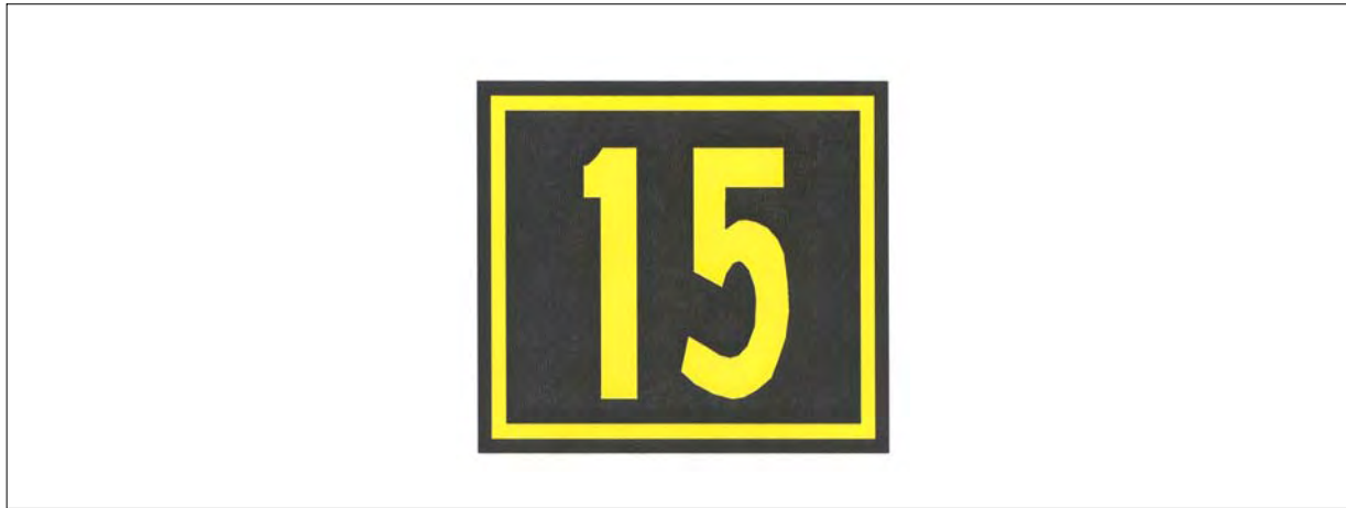
FIG AD 1.1-41 Runway Location Sign
