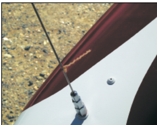
Figure 18-7. A string simply tied near the nose of the gyroplane that can be viewed from the cockpit is often used to indicate rotation about the yaw axis. An inclinometer may also be used.
