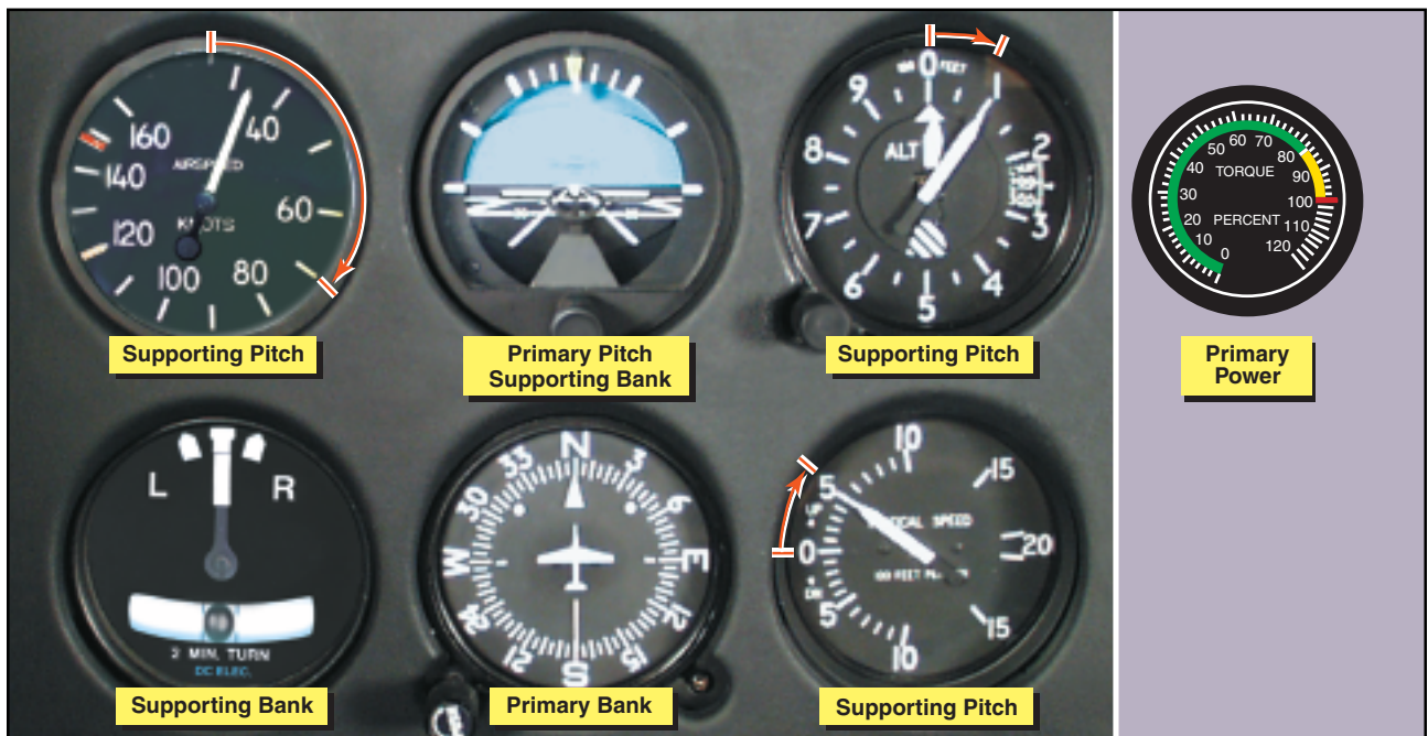
Figure 12-22. Flight instrument indications during an instrument takeoff.
