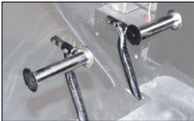
Figure 4-5. Antitorque pedals compensate for changes in torque and control heading in a hover.
