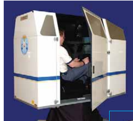
Spatial Disorientation (Vertigo) Demonstrators. Above: GYRO-2 General Aviation Trainer. Right: Virtual Reality Disorientation Demonstrator.
