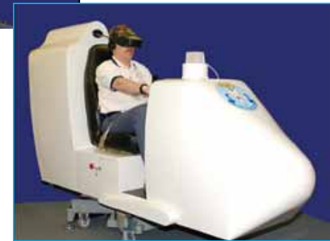
Spatial Disorientation (Vertigo) Demonstrators. Above: GYRO-2 General Aviation Trainer. Right: Virtual Reality Disorientation Demonstrator.
