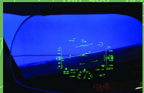
The FAA and industry are pursuing use of enhanced flight visibility systems to achieve "equivalent visual operations".
