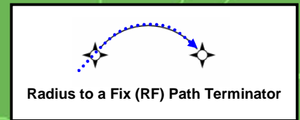
Advanced features such as RF path terminators allow for the design of procedures that deliver measurable benefits to those operators equipped to execute them.
