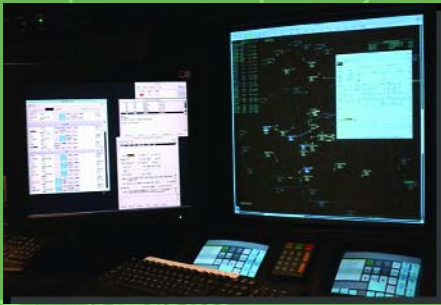
ATOP has been implemented in New York and Oakland Air Route Traffic Control Centers (ARTCC). ATOP Ocean21 system (pictured here) supports reduced separation standards for RNP-approved aircraft.
