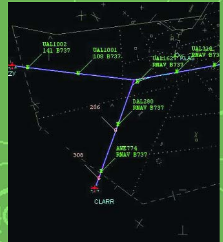
Future ground-based tactical controller tools will assist the controller with compression management and merge points, to maintain efficient flow into the airport.
