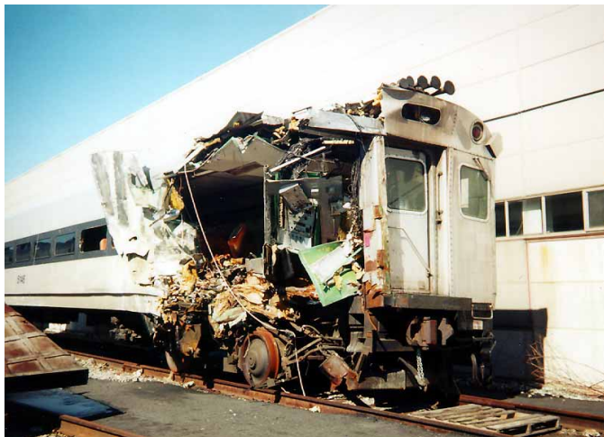
Figure 1: Photograph of the Cab Car Damaged in the Secaucus, New Jersey Accident [1].
