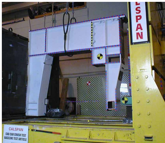
Figure 9: Quasi-Static Test Setup
