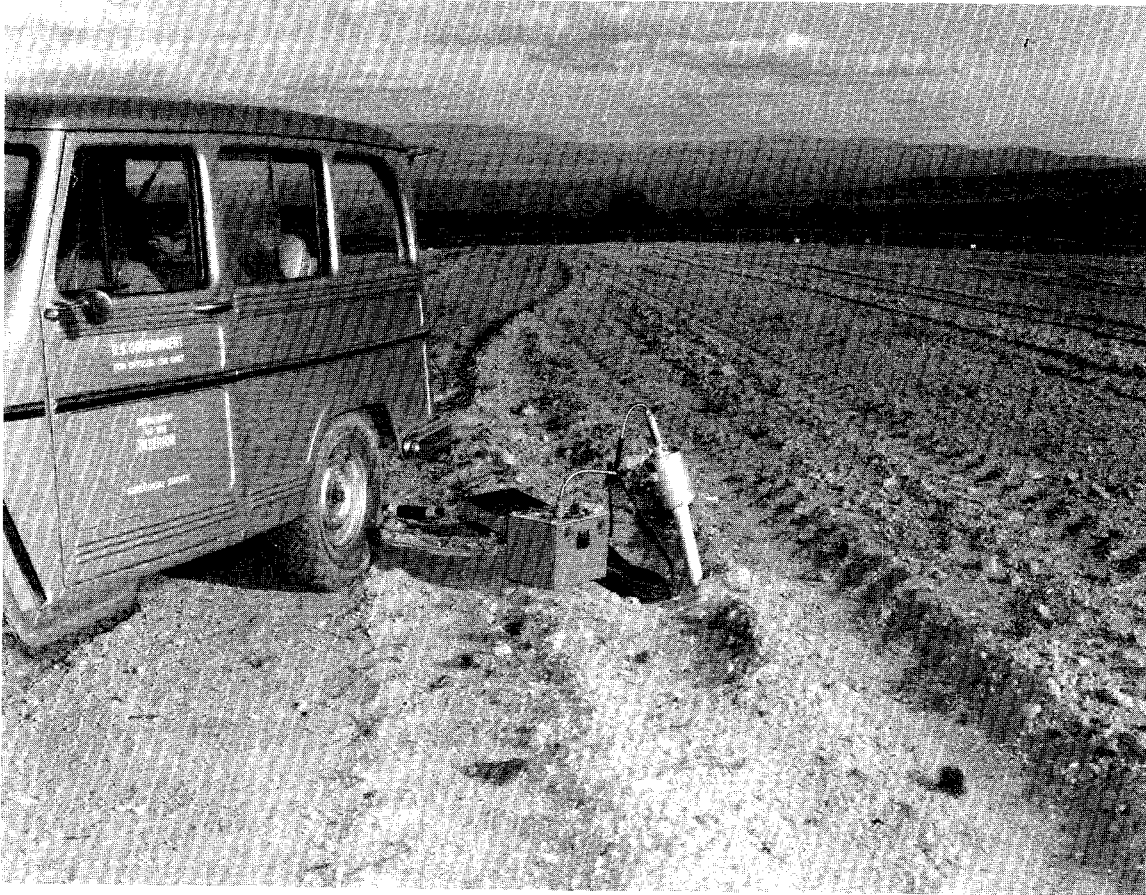
Fig. G-20. Measuring moisture levels in Pit 2, Area G with a neutron depth moisture gage.
