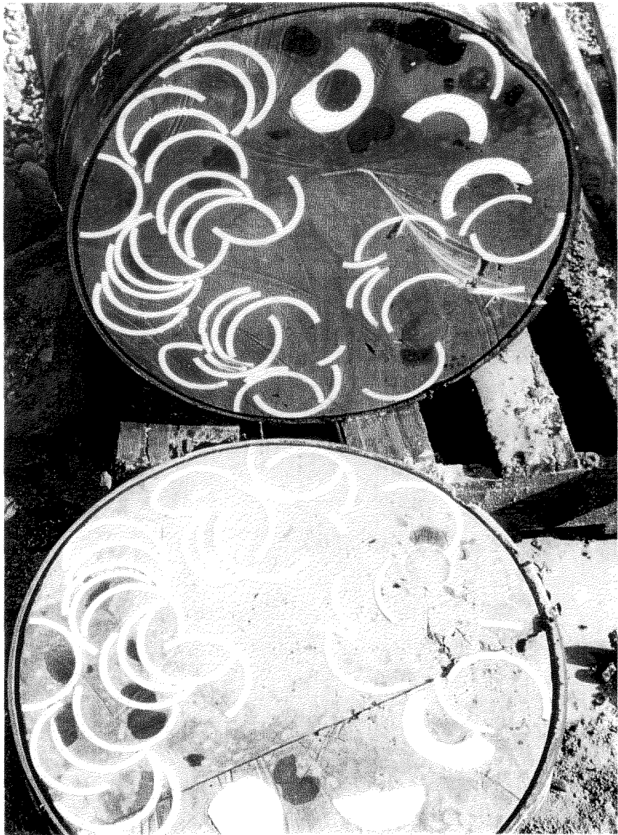
Figure B-6. Penetrated simulated waste containers with grouted contents.
