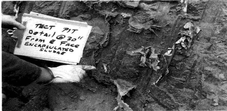
Figure B-7. Effective grouting results for simulated oil sludge at the Idaho National Engineering and Environmental Laboratory.
