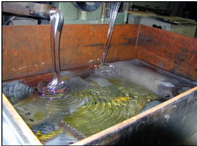
Figure 3-1. Macroencapsulation of Hazardous Debris
