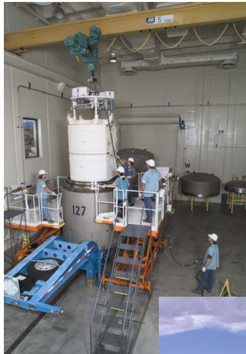
Readying TRU waste drums and installing into TRUPACT II containers
