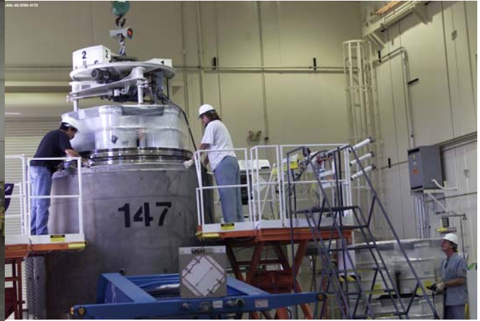
Readying TRU waste drums and installing into TRUPACT II containers
