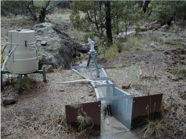
Storm water sampling stations
