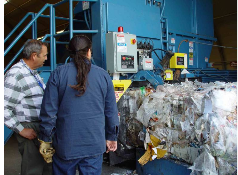
LANL baling machine creates wired, 1600 lb. bales using 2800 psi of pressure.
