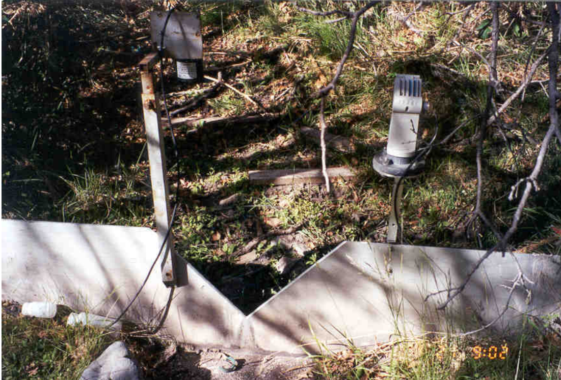
Figure 4.1-2. SWSC Spring V-notch weir. SWSC Spring has been dry since December 2001. Photo was taken June 2002.
