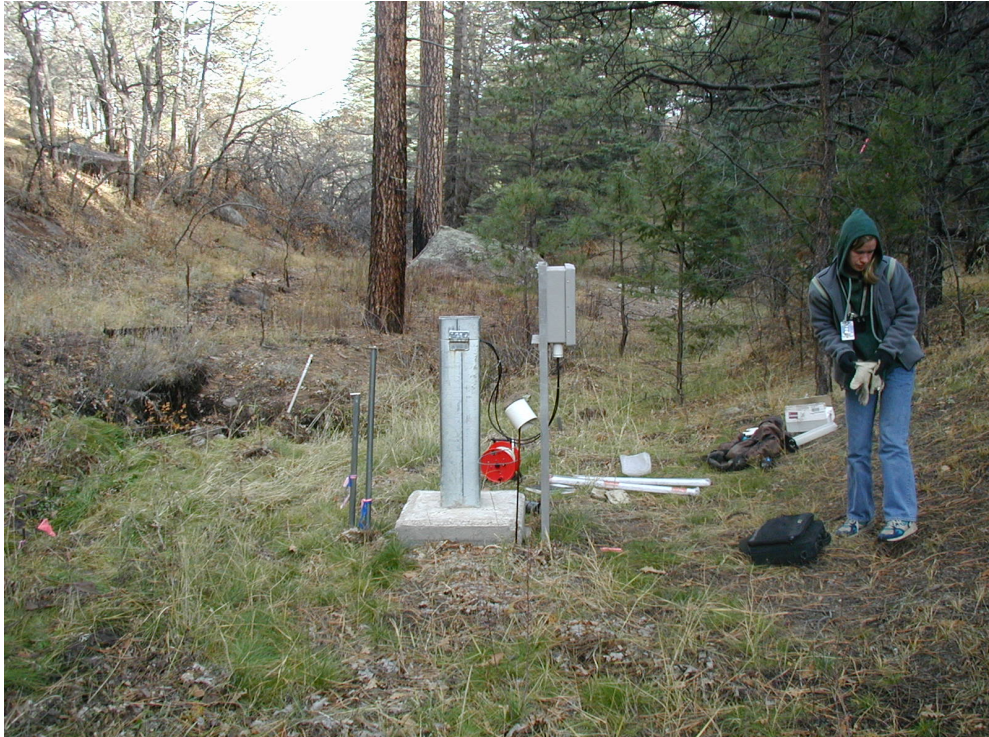
Figure 3.3-4. Field personnel conducting monthly field measurements at Well 16-02658 in Cañon de Valle. Photo was taken in November 2002. View is looking down canyon. A piezometer nest (Locations 16-02459 and 16-02460) is also visible to the left of the well housing.
