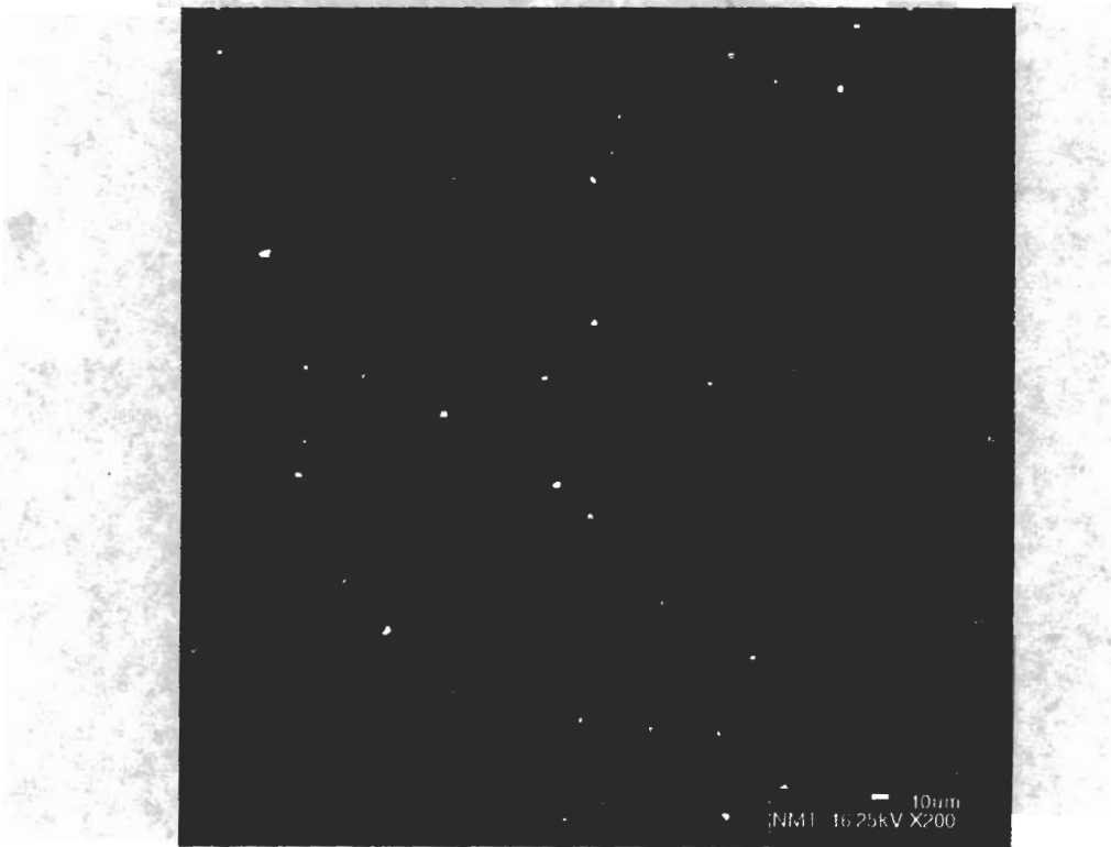
Photograph 11. SEM image of homogenous glass
