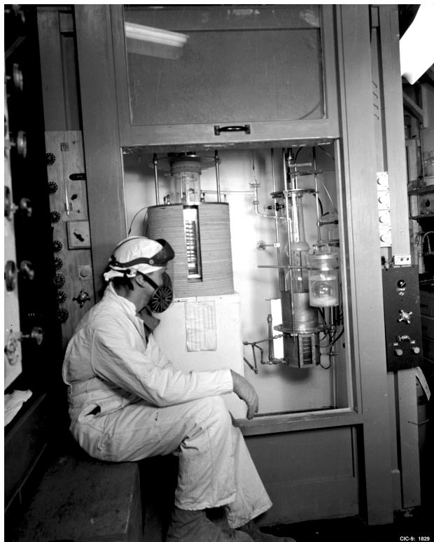
Figure 44. An early plutonium worker performs a purification operation in an open chemical hood.
