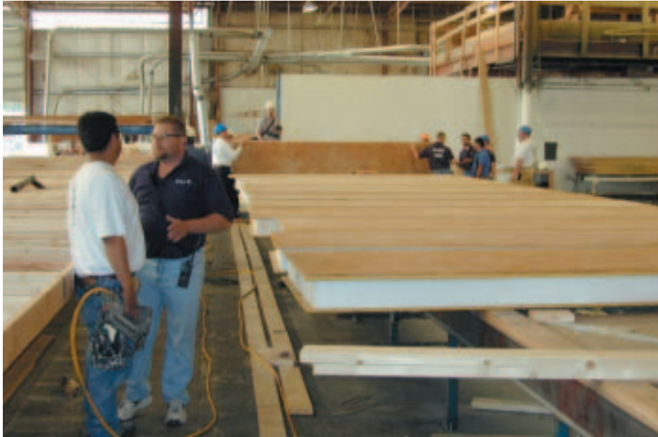
SIPs can be faced with wood sheathing made from certified wood.
