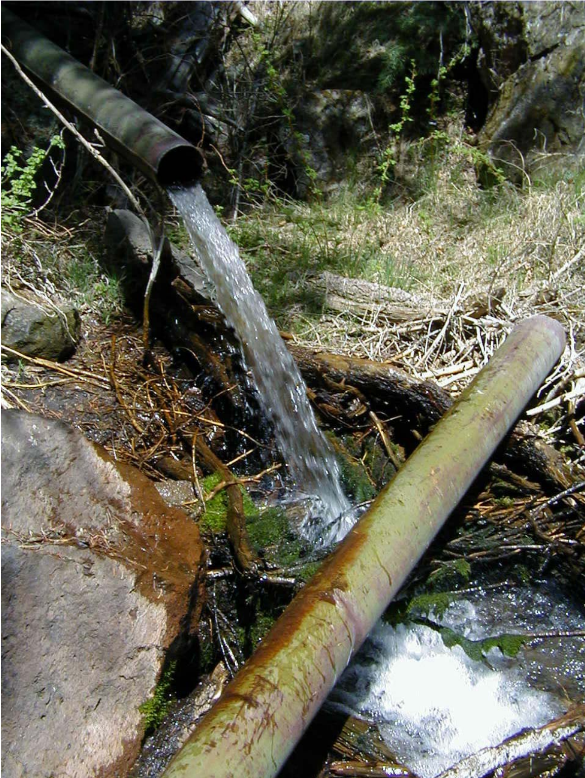
Figure E.11-2. Photograph of disconnected discharge pipe from Water Canyon Gallery taken April 27, 2000; the temperature is 14°C, and the flow rate is 120 L/min ( \pm 25\% )
