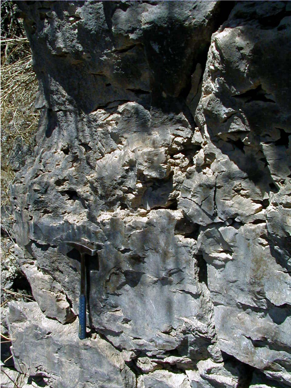
Figure E.11-3. Photograph of vesicular cavities in a flow unit of densely welded Tshirege Member, Bandelier Tuff, about 10 m above the entrance to Water Canyon Gallery
