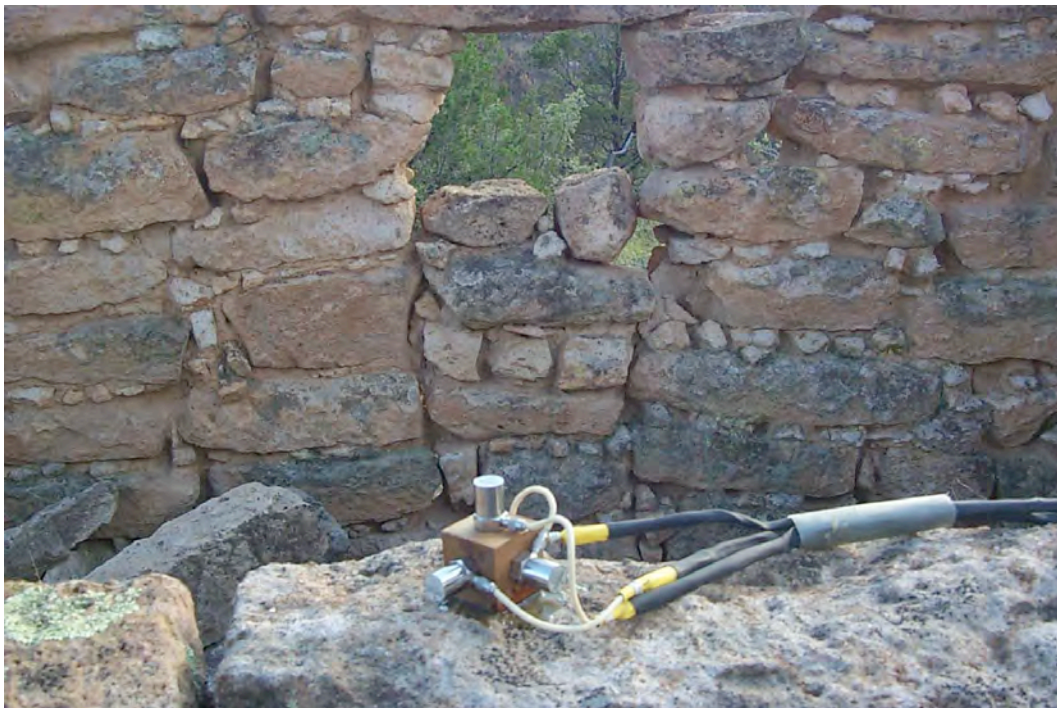
Figure 20.4. This vibration sensor sits on the top of a standing wall at Nake'muu.
