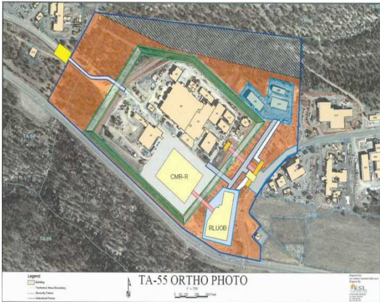
Figure 6-4. The extent of the work to be done at TA-55. The blue line represents the outermost fence perimeter. The orange layer represents the riprap rock field, and the green layer is the new PIDADS.
