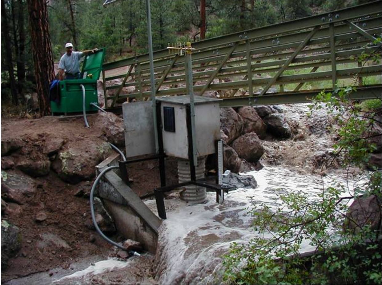
Storm runoff monitoring station on LANL, DP Canyon.
