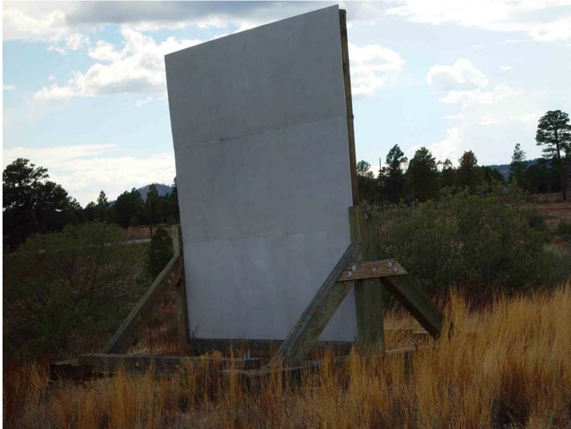
Figure 8: This aluminum-covered board is used to calibrate a CO2 laser LIDAR system located at TA-33. It is located along the dirt road to Tract 49C.
