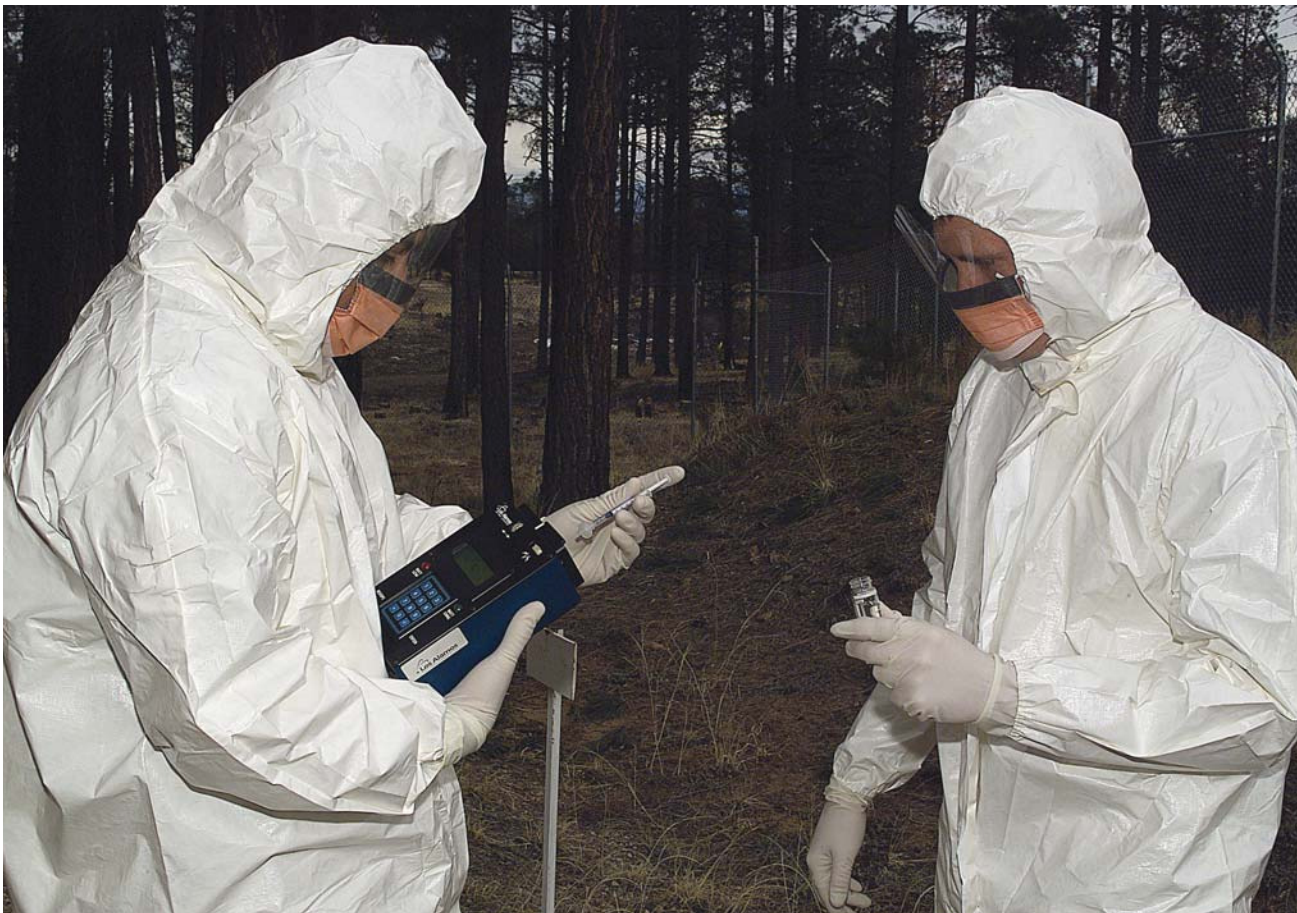
A training exercise, using ROB (Reagentless Optical Biosensor) to test environmental samples
