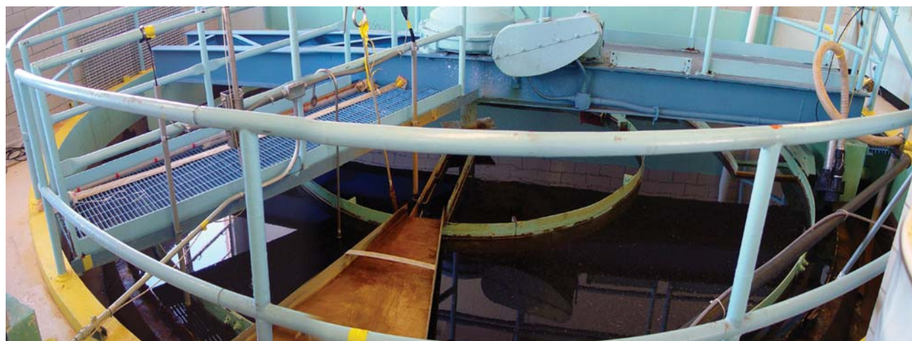
Initial treatment of radioactive liquid waste by chemical precipitation
