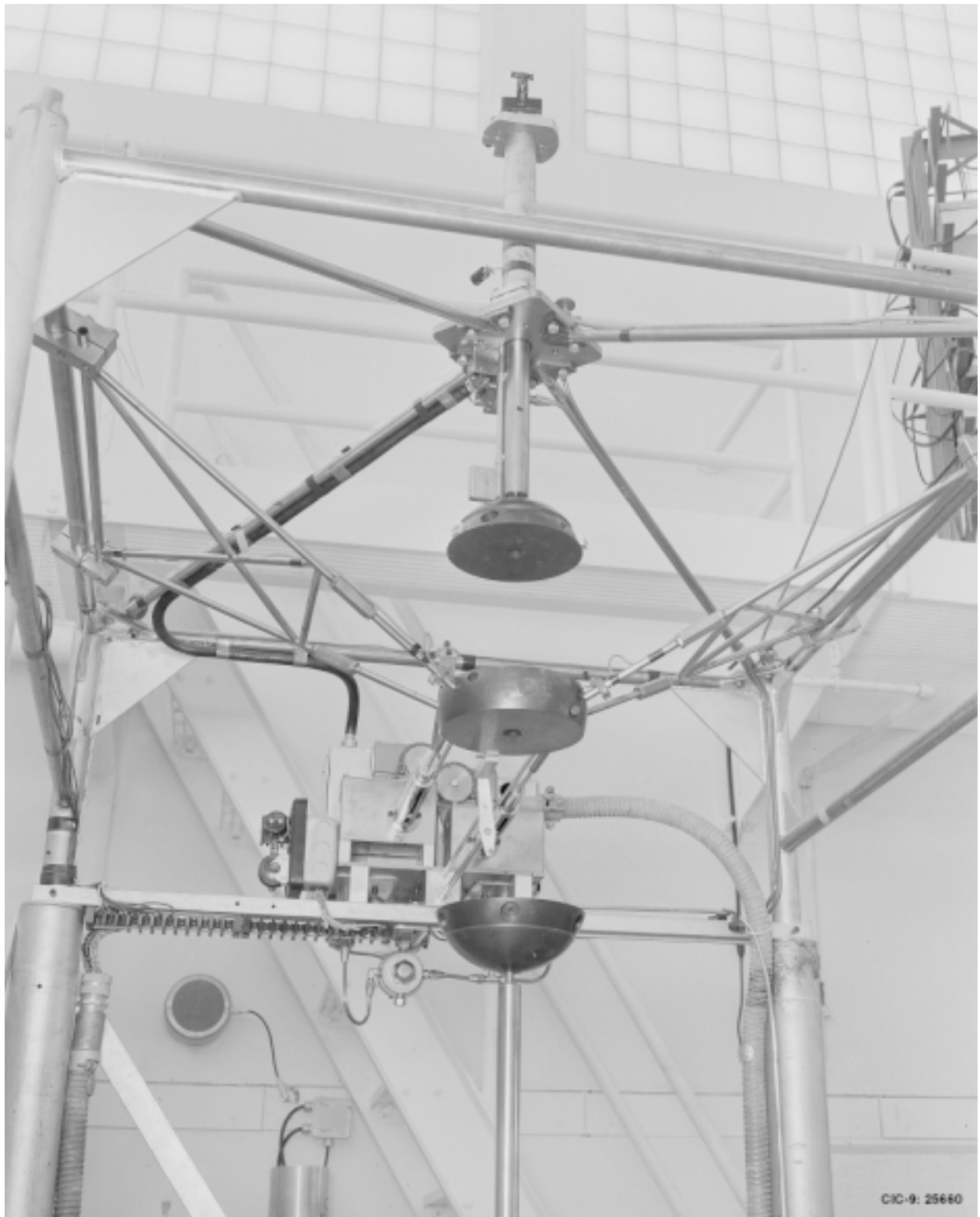
Figure 48. The Los Alamos Scientific Laboratory Lady Godiva assembly (unreflected enriched-uranium sphere) in the scrambled configuration.
