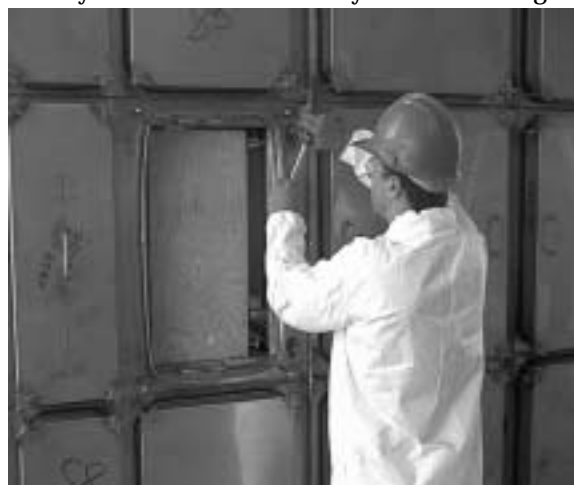
Figure 6.9 – Using Wrench to Operated Four-Bar-Linkage Gasket Seal Clamping Mechanism
