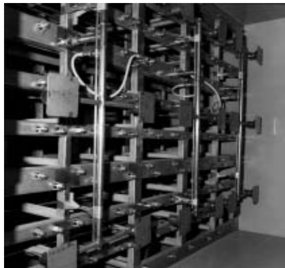
Figure 4.16 – Absorber Mounting Frame with Test Section Manifold
