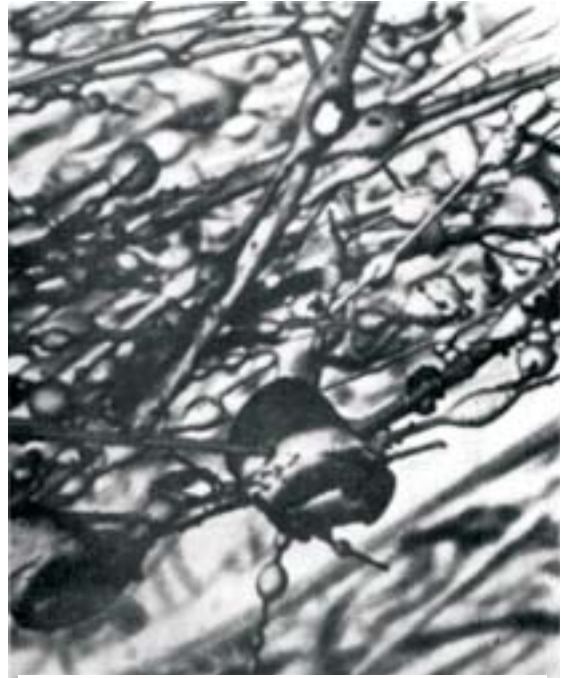
Figure 10.5 – Scanning Electron Micrograph of HEPA Filter Media Loaded with Smoke Aerosols from Composite Crib Fires. (Note: the drop-like globules attached to the filter fibers that suggest the liquid nature of the aerosol) 17
