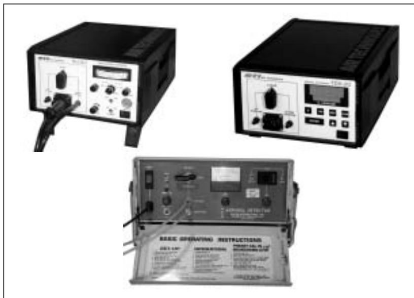
Figure 8.6 – Commercially Available Packaged Forward-light Scattering Photometer for HEPA Filter In-place Testing
