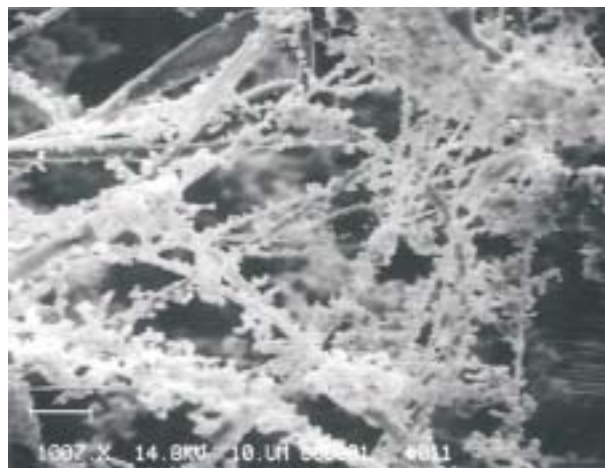
Figure 10.6 – Scanning Electron Micrograph of Sodium Chloride Aerosols on Glass Fiber Prefilter. 18
