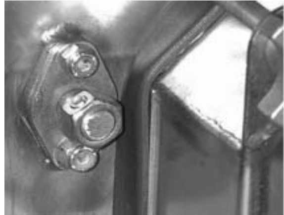
Figure 6.10 – Filter Locking Mechanism Drive Bolt Located at the Front Exterior of the Housing
