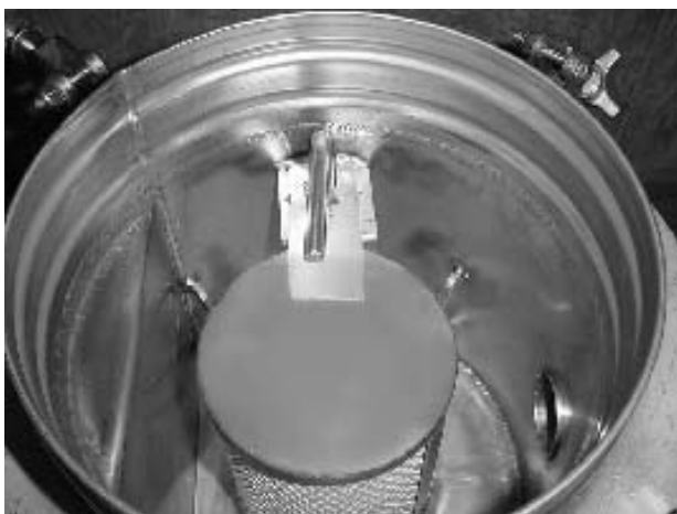
Figure 6.25 – Clearance Between Radial Flow Filter and Housing
