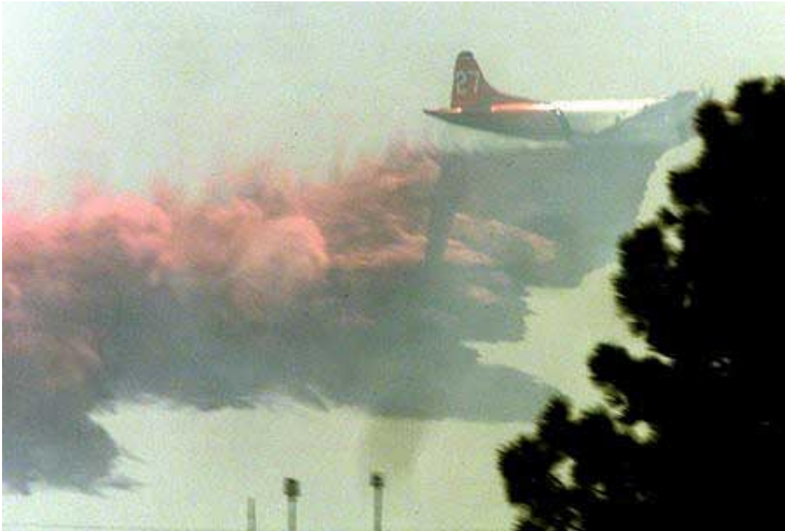
PHOTO 2.1— Slurry Being Dropped
